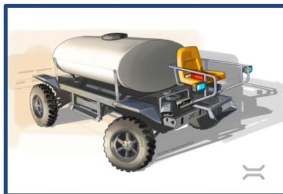
commercial orchard pull-rig agricultural spray trailer. Electricore will oversee the demonstration at Tech Agricultural's farms outside of Buttonwillow, in Kern County. The vehicle will operate autonomously based on robotics developed by the Robotics Institute at Carnegie Mellon University.
