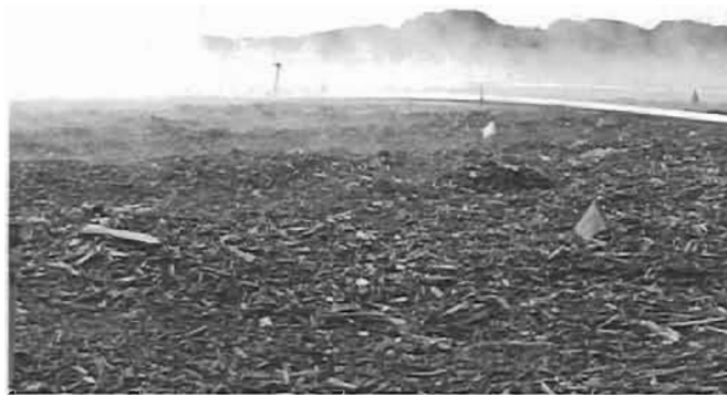
Normal operation results in a steamy surface on the biofilter (above photo from SKIC)
