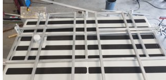
Folded Railing system for Transport
