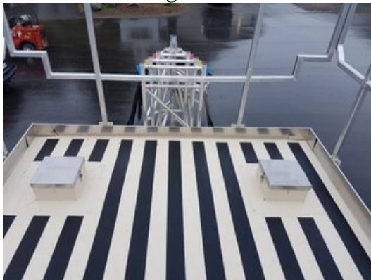
OSHA railing with Toe Board
