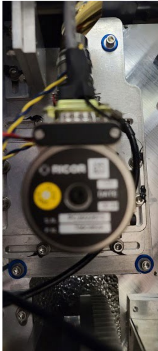
Figure 6. Image showing baseplate and screws with rubber grommets.
