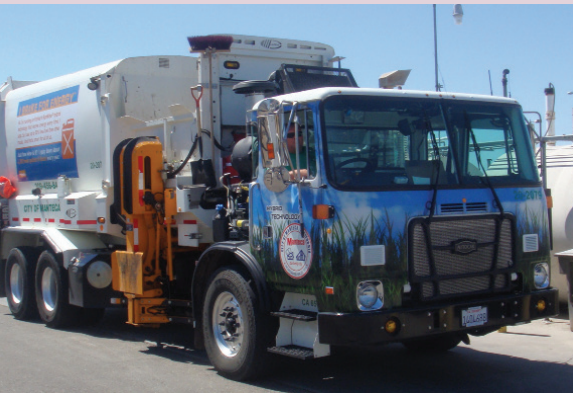
The city of Manteca’s hybrid hydraulic refuse trucks were developed through the Technology Advancement Program.
